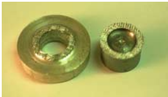
Fig. 7 Explosive Clad Ram Tensile Specimen
