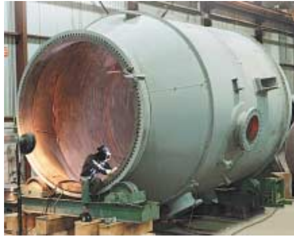
Fig. 9 Titanium Clad SA-516-70 Carbon Steel Reactor Component for Production of PTA
