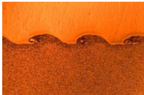
Fig. 4 Titanium to Carbon Steel Explosive Bond Photo courtesy Clad Metal Products
