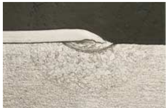
Fig. 1 Tantalum (0.5 mm, .020") Welded to Titanium
