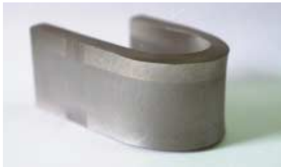
Fig. 6 Explosive Clad Side Bend Test Specimen
