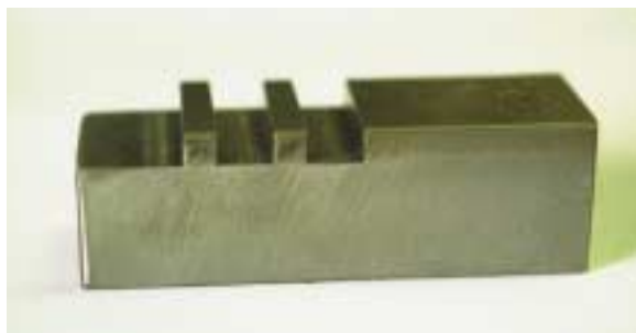
Fig 5 Explosive Clad Shear Test Specimen
