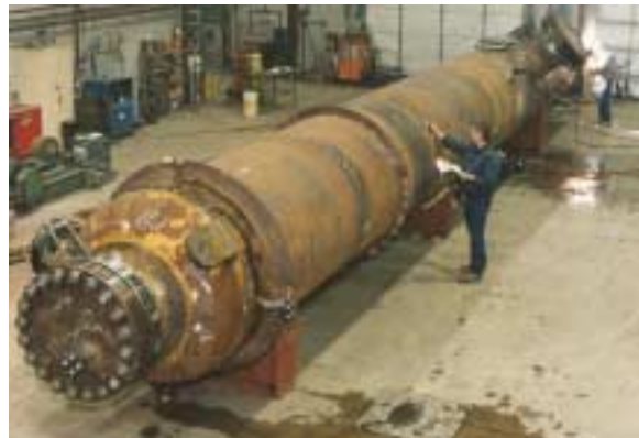
Fig.10 Titanium Clad Carbon Steel Reactor, 1/8" Grade 1 on SA-516-70 for Production of Organic Chemicals.
