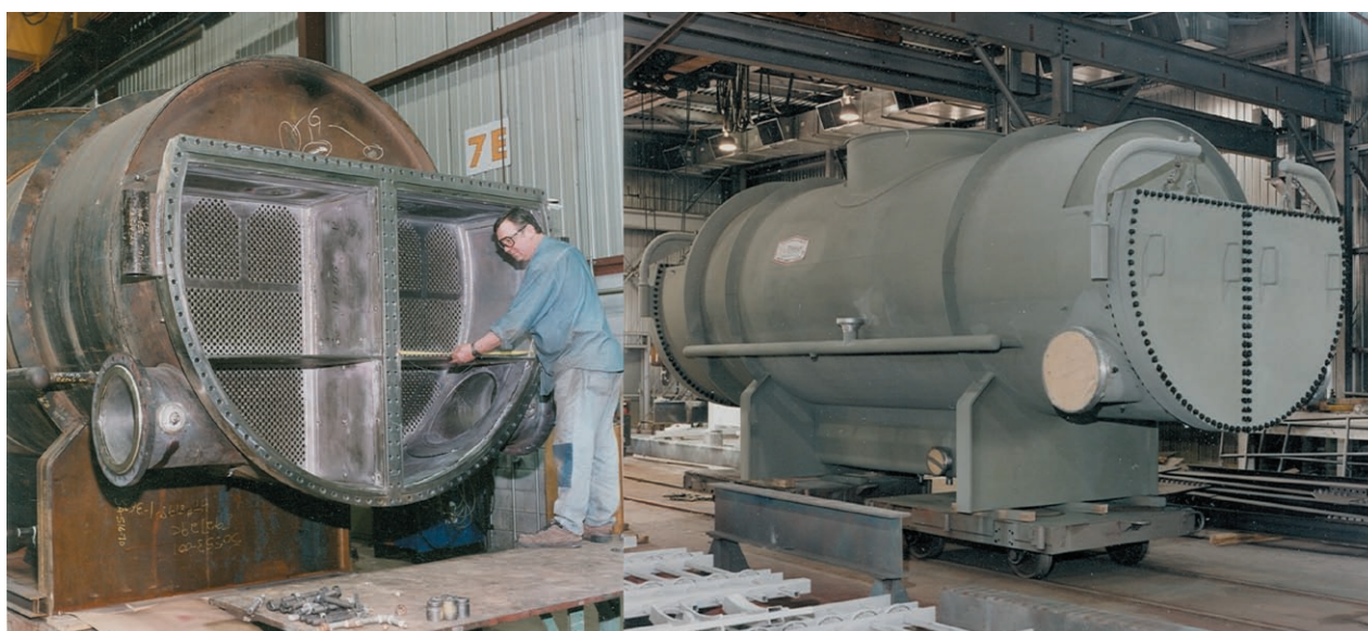
Figure 3. Steam surface condensers for refineries.
